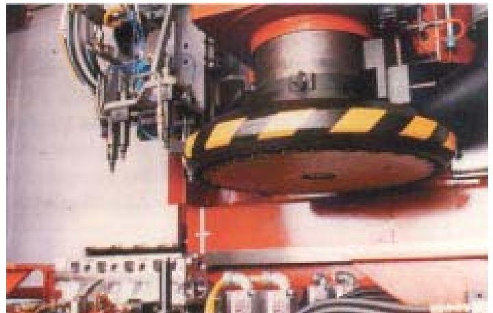
Figure 23 -30 HP 5,000 RPM facemilling spindle (Turchan1991)
