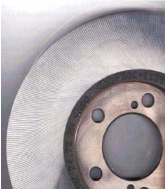
Figure 33 - Cast iron brake rotor finish milled with CBN at 7,000 SFM
